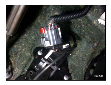
With everything now connected, be sure that the Sprint Booster and OEM harness do not interfere with your foot and the pedal. Using the zip tie supplied you can strap it up out of the way.
