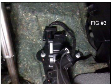
Step 4- Plug the male end of the Sprint booster into the factory Mustang pedal. You will hear it click in place. It will look as FIG #3. While paying attention not to tangle wires, plug the Mustang harness that used to be plugged into the pedal now into the female end of the Sprint booster. In short, you have put the Sprint Booster inline of the OEM factory connection, as FIG #3B displays.
