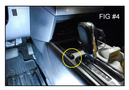
Again be sure that the wire to the button is out of the way of your leg or foot. It is wise to route it under dash panels to prevent it from catching on any foreign objects moving in the car. Another zip tie may be needed to aid in doing so.
